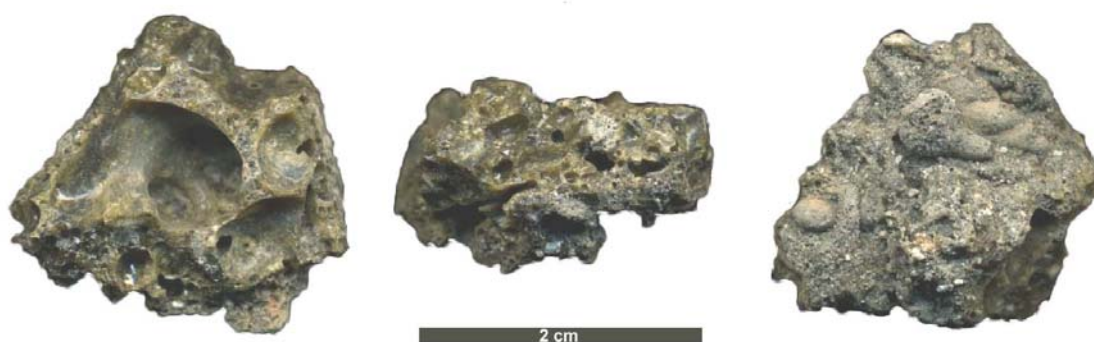
Fig. 2. A specimen of atomsite from Semipalatinsk test site. Left: top side. Middle: edge. Right: bottom side. Mass: 2,545 g.
