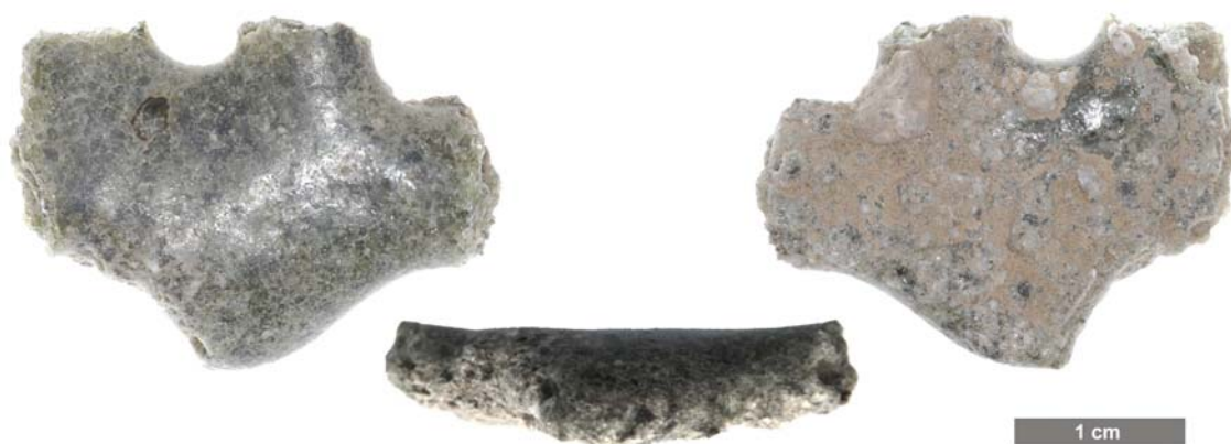
Fig. 1. A specimen of Trinitite. Left: top side. Middle: edge. Right: bottom side. Mass 3.170 g.
